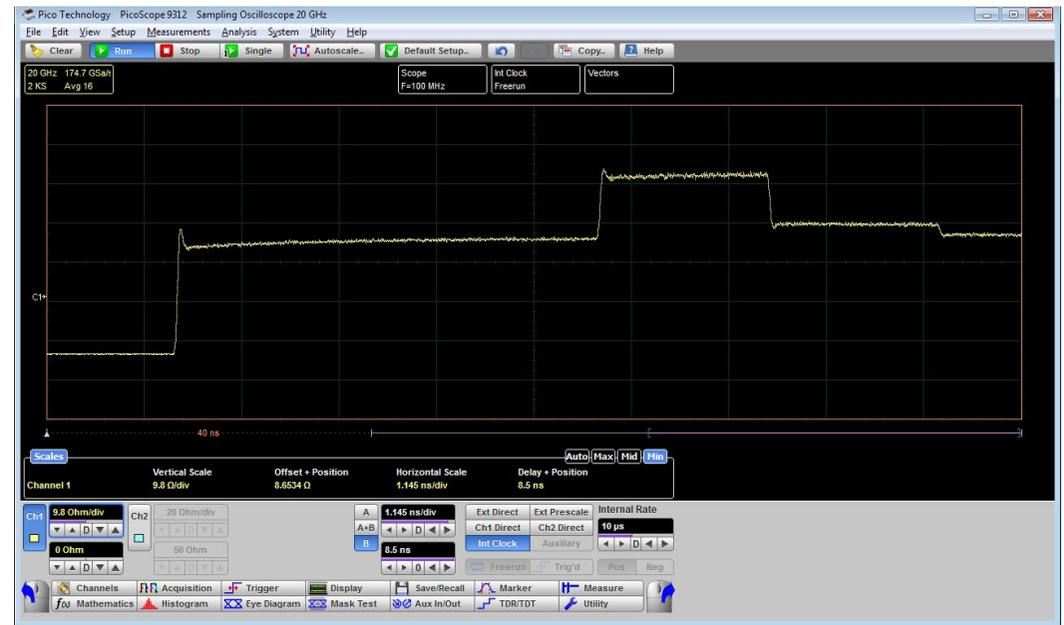
The PicoScope 9311-15 and 9311-20 generate 2.5 to 7 V steps with 60 ps rise time from built-in step recovery diodes. They are supplied with a comprehensive set of calibrated accessories to support your TDR/TDT measurements, including cables, signal dividers, adaptors, attenuator and reference load and short.
