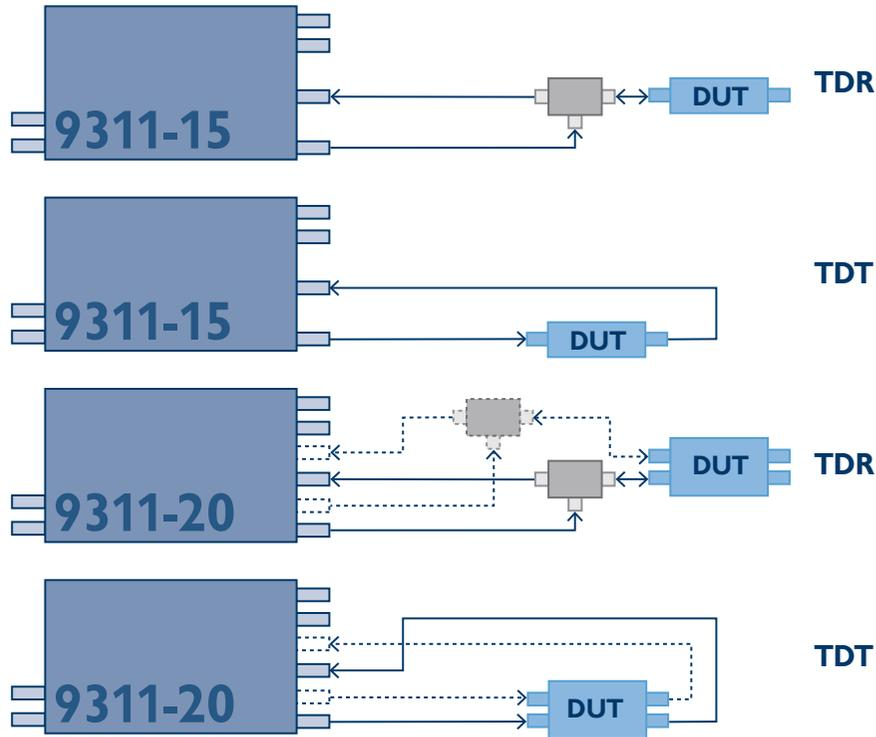
Connection diagrams: PicoScope 9311 sampling oscilloscopes in use with devices under test (DUT) in TDR and TDT applications
