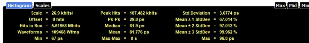
Histograms can be constructed on waveforms on either the vertical or horizontal axes. The most common use for a vertical histogram is measuring and characterizing noise and pulse parameters. A horizontal histogram is typically used to measure and characterize jitter.
